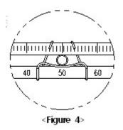
If connection bar does not point at 50% point, then adjust bracket or feedback link bar position. Failure to position at 50% would lower the linearity of the positioner.
